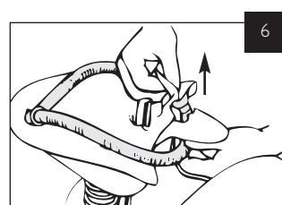
Slide tubing through slot in lung plate, to detach airway assembly.
