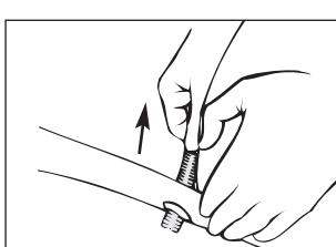
Pull expiration tube from its retainer in the manikin's side.
