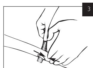
Push expiration tube into retainer in manikin's side until end protrudes about 2-3 cm (1").
