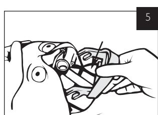
Install jaw by sliding its forked portions over steering pins in the inner head.
